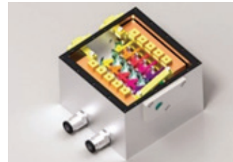
Palm-sized (about 1/25 compared to conventional models) photonic crystal laser module (prototype)
